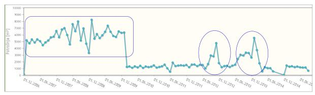
Figure 8: Increased water consumption due to cracked water pipes in the water distribution system outside a public building detected by EMIS
